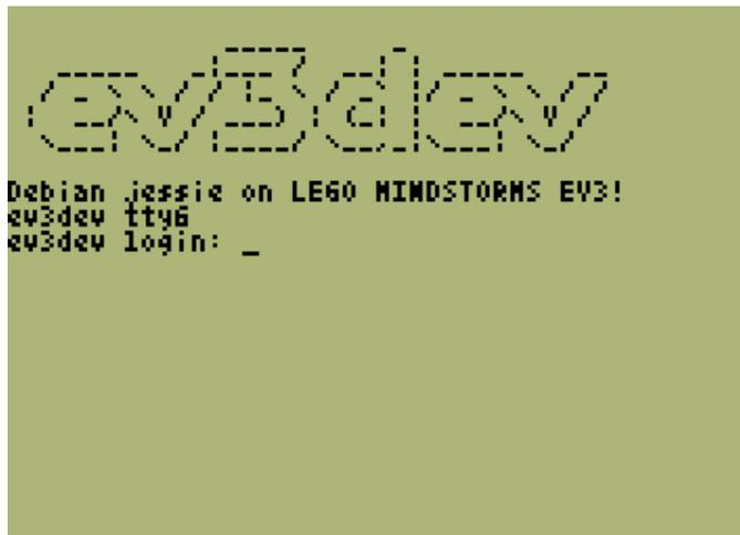
Figure A.12: The EV3 screen once the terminal has been changed with the `chvt 6` command
