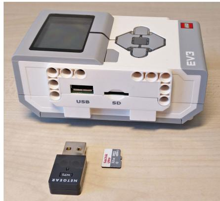
Figure A.2: A SanDisk 32 GB HC MicroSD and a Netgear N150 - WNA1000 Wi-Fidongle in front of their respective ports on the EV3.
